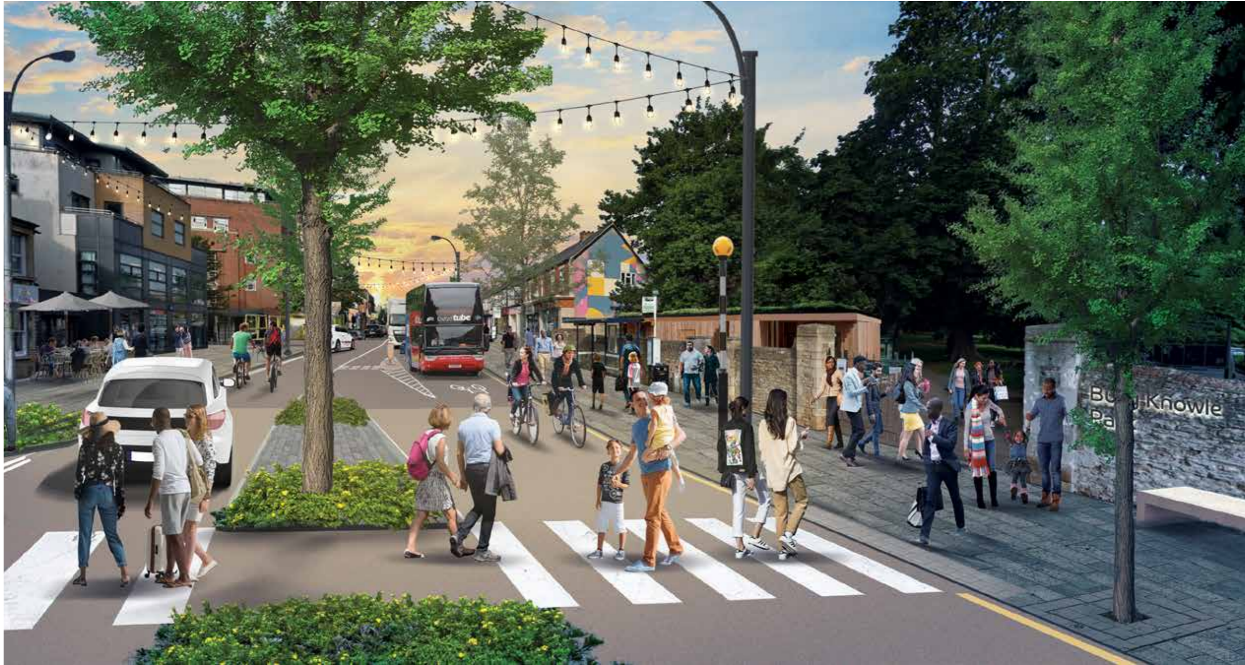
Conceptual visualisation of how the eastern gateway might look, with bus stopping and movement improved, new central median feature and surfacing, feature lighting, improved pedestrian crossing, and enhanced public realm at Bury Knowle Park entrance (View west along London Road from outside Bury Knowle Park entrance)
