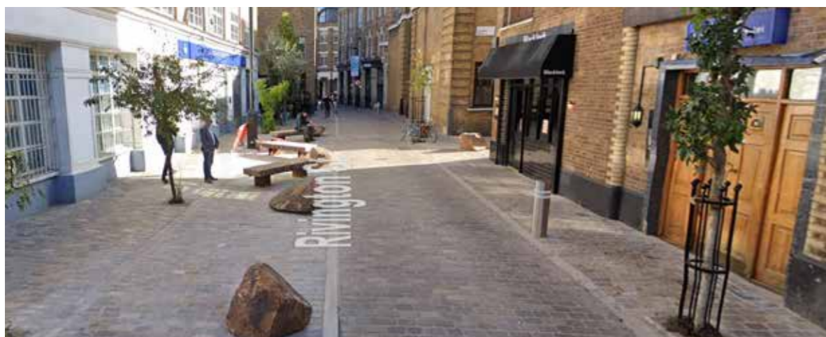
Example of pocket plaza created by widening pavement space while still allowing vehicular access, and incorporating tree planting and seating (Shoreditch, London)
